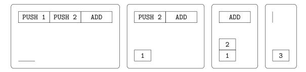
FIGURE 5.1. Evaluation of a stack-based program that adds 1 and 2. Each state is presented in a rounded rectangle, and is a combination of a program and a stack. The program is presented horizontally at the top of the state, with the operations to be evaluated from left to right. The stack is presented vertically at the bottom of the state, growing upwards. The evaluation of the program proceeds from left to right.
