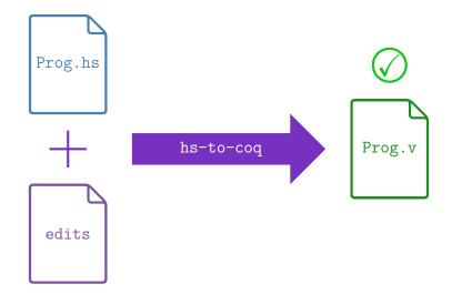
FIGURE 1.1. How hs-to-coq operates: Given a Haskell file (Prog.hs), the user writes edit files (edits) which record the changes that will be made to the generated output. Once they have both of these, the user feeds them into hs-to-coq, examines the generated Coq output (Prog.v), and proves it correct.
