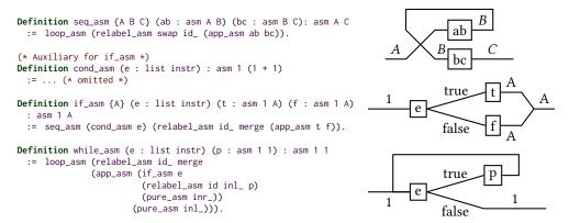
Fig. 17. High-level control flow in Asm
