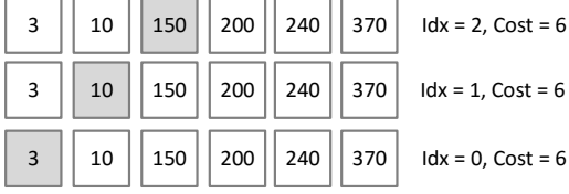
FIGURE 2—A client wishing to retrieve an item with label “3” from a server holding a sorted list of 6 items would need to perform three rounds of probing. During each probe, the client guesses an index, uses PIR to retrieve the (label, c) -tuple at that index, and refines the guess accordingly. “Cost” indicates the number of items processed by the server in each probe.
