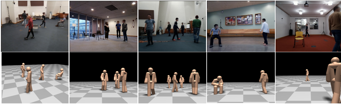
Figure 1-2: Through-Wall 3D Human Pose Estimation. RF-Pose3D estimates 3D human skeletons for multiple people and in different environments. It captures depth information in addition to the 2D human poses. Top: Images captured by cameras for visual reference. Bottom: Predicted 3D human poses with RF signals only. Full video is available at: https://www.youtube.com/watch?v=XCEgyQKLaJ0 .
