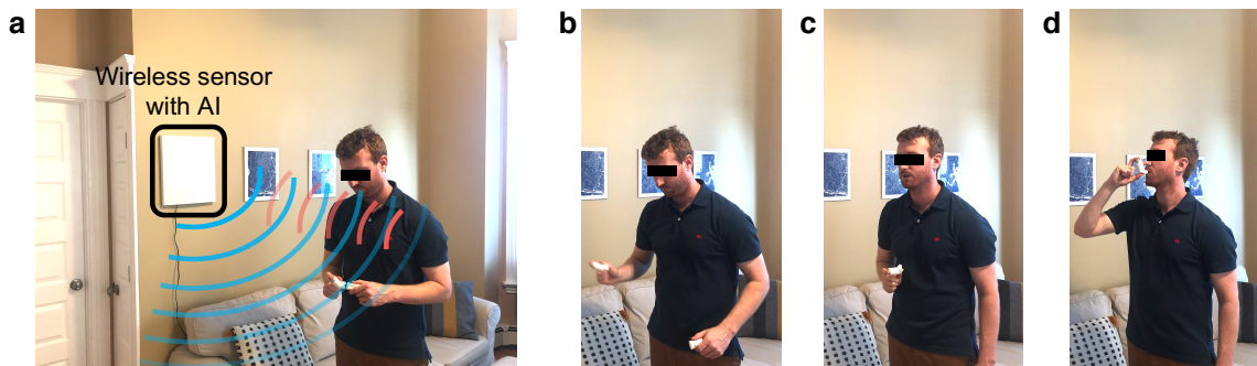
Figure 6-1: A use case illustration of the wireless AI-based system to monitor individual MSA with an inhaler device. a , The wireless sensor is mounted on the wall, analyzing the surrounding radio signals using AI. The AI solution would detect when the person started to use an inhaler. b–d , Our AI solution also tracks the motion during the MSA event and detects that the person shook the device, exhaled before use and, finally, inhaled a dose. (We obtained informed consent from the participant for the use of his photographs.)
