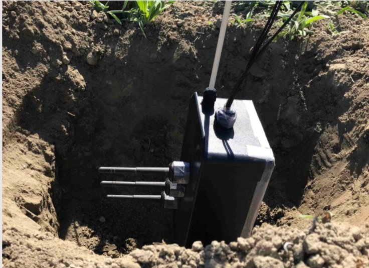
Waterproof box holding the RX antenna array
