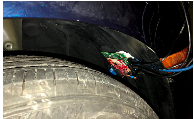
Figure 9: Osprey was also evaluated on a passenger car. Osprey’s hardware is shown to be mounted in the tire well of a 2019 Honda Odyssey.
