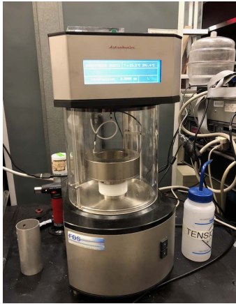
Figure 10: Digital tensiometer with a resolution of 0.1mN/m for measuring ground truth of surface tension (Model: Dataphysics DCAT 11 [15])
