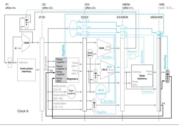
**FIGURE 4.12.15 Clock cycle 9.** The WB stage writes the sum in MEM/WB into register \$14, completing add and the five-instruction sequence. The instructions after add are shown as inactive for pedagogical reasons.
