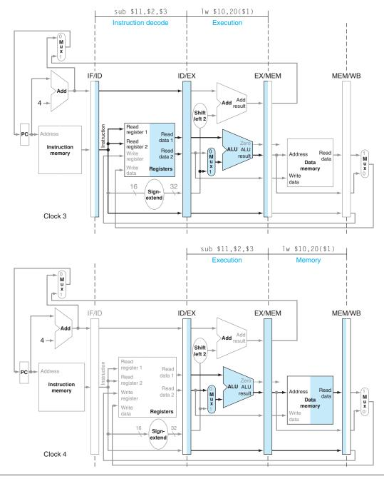
**FIGURE 4.12.9** Single-cycle pipeline diagrams for clock cycles 3 (top diagram) and 4 (bottom diagram). In the third clock cycle in the top diagram, ]w enters the EX stage. At the same time, sub enters ID. In the fourth clock cycle (bottom datapath), ]w moves into MEM stage, reading memory using the address found in EX/MEM at the beginning of clock cycle 4. At the same time, the ALU subtracts and then places the difference into EX/MEM at the end of the clock cycle.
