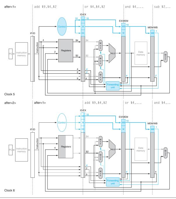
**FIGURE 4.12.17 Clock cycles 5 and 6 of the instruction sequence on page 4.12-26.** The forwarding unit is highlighted when it is forwarding data to the ALU. The two instructions after add are shown as inactive just to emphasize what occurs for the four instructions in the example. The bold lines are those active in a clock cycle, and the italicized register numbers in color indicate a hazard.
