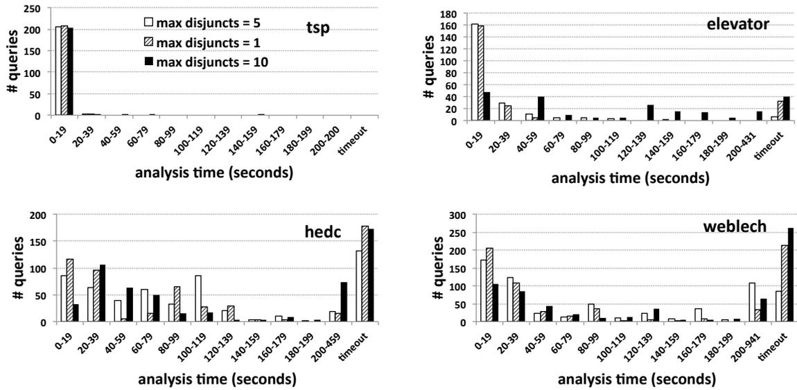
Figure 13. Running time of thread-escape analysis per query for different degrees of underapproximation  $k = 1, 5, 10$  in its meta-analysis on our smallest four benchmarks. The timeout columns denote queries that could not be resolved in 1,000 minutes. Setting  $k$  to 1 or 10 resolves fewer queries than  $k = 5$  for the shown benchmarks and also caused the analysis to run out of memory for the largest three benchmarks.
