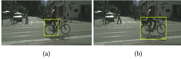
Fig. 12. A violation of the high-velocity constraint where Figures 12a and 12b are two continuous frames from the CITYSCAPES dataset. The predicted bounding boxes in these two frames are inconsistent in their positions and sizes, thus exaggerating the speed of the object.
