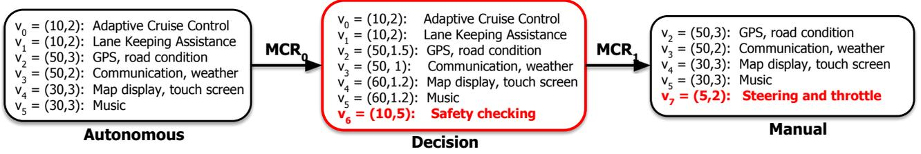
Fig. 4: Multi-mode system case study. Here, each  $v_i = (P_i, B_i)$  gives the period  $P_i$  and WCET  $B_i$  (in ms) of the task  $v_i$ .
