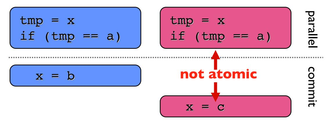
Synchronization, e.g. lock(), must happen in serial mode
