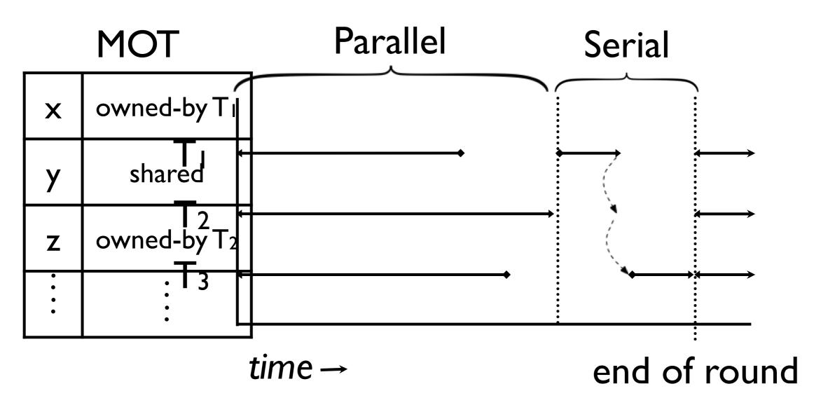
**Parallel mode:** no communication (can write only to private data) **Serial mode:** arbitrary communication
