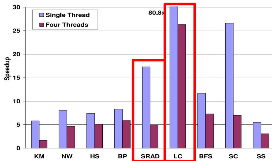
Fig. 2. The speedup of the GPU implementations over the equivalent single- and four-threaded CPU implementations. The execution time for calculating the speedup is measured on the CPU and GPU for the core part of the computation, excluding the I/O and initial setup. Figure 4 gives a detailed breakdown of each CUDA implementation's runtime.
