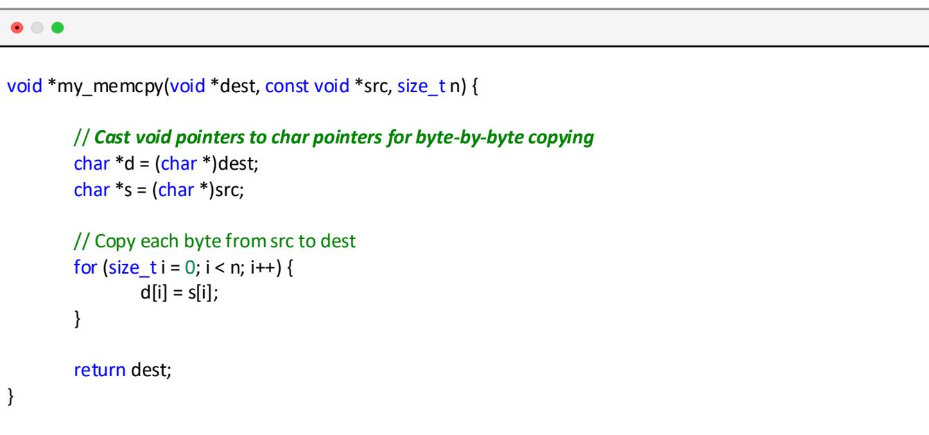
The screenshot shows a code editor window with three tabs at the top. The active tab contains the following C code:
