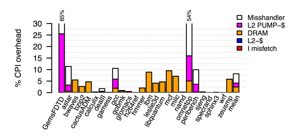
Simulated Alpha+PUMP running SPEC2006 benchmark suite with composite micro-policy (memory safety + CFI + taint tracking)
