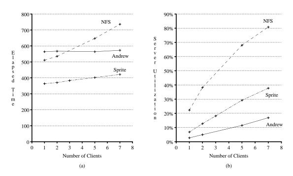
**Figure 5.** Performance of the Andrew benchmark on three different file systems; Sprite, Andrew, and NFS. (a) shows the absolute running time of the benchmark as a function of the number of clients executing the benchmark simultaneously, and (b) shows the server CPU utilization as a function of number of clients. The Andrew and NFS numbers were taken from [HOWA87] and are based Sun-3/50 clients. The Sprite numbers were taken from Table 6 and Figure 4 and re-normalized for Sun-3/50 clients.
