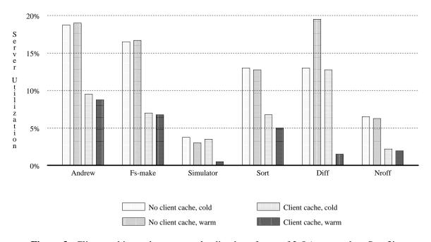
**Figure 3**. Client caching reduces server loading by a factor of 2-5 (measured on Sun-3's with variable-size client caches).
