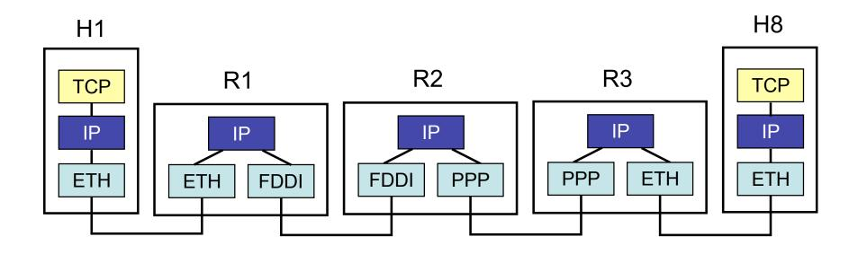
Example of protocol layers used to transmit from H1 to H8 in network shown on previous slide.
