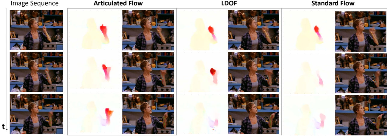
Figure 3. Articulated flow. Left : A video sequence ordered in time with fast rotations of left lower arm. Right : Motion flow is displayed as a) color encoded optical flow image, and b) the warped image using the flow. We compare the proposed articulated flow, Large Displacement Optical Flow (LDOF) [5] and coarse-to-fine variational flow of [4]. The dashed lines in the warped image indicate the ideal position of the lower arm. If the flow is correct, the warped arm will be aligned on the dashed line. Standard optical flow cannot follow fast motion of the lower arm in most cases. LDOF, which is descriptor augmented, recovers correctly in case of correct descriptor matches. However, when descriptors capture the hand but miss the arm, hand and arm appear disconnected in the motion flow space (2nd row). Knowing the rough body articulation points allows to restrict our motion model to be a kinematic chain along the body parts. The resulting articulated motion flow is more accurate.
