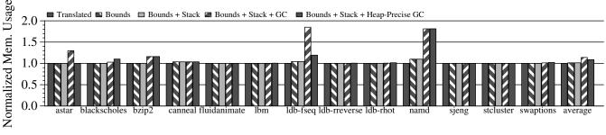
**Figure 10.** Normalized memory usage for Ironclad C++ code with (from left to right) bounds checking metadata, bounds and stack checking metadata, both metadata with conservative GC, and both metadata with heap-precise GC.
