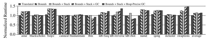
**Figure 9.** Normalized runtimes for refactored Ironclad C++ code with (adding checking from left to right): no checking, bounds checked arrays, safe stack allocations, safe heap allocations, and heap-precise garbage collection.
