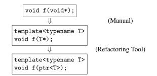
**Figure 8.** Common refactoring to remove void\* pointers. First we manually add templates. Then the refactoring tool adds ptrs.
