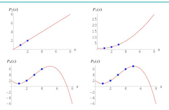
The Lagrange interpolating polynomial is P(x) that passes through n points:  $(x_1, y_1 = f(x_1)), \dots, (x_n, y_n = f(x_n))$
