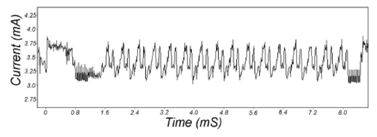
• This figure shows simple power analysis of DES encryption. The 16 rounds are clearly visible.
