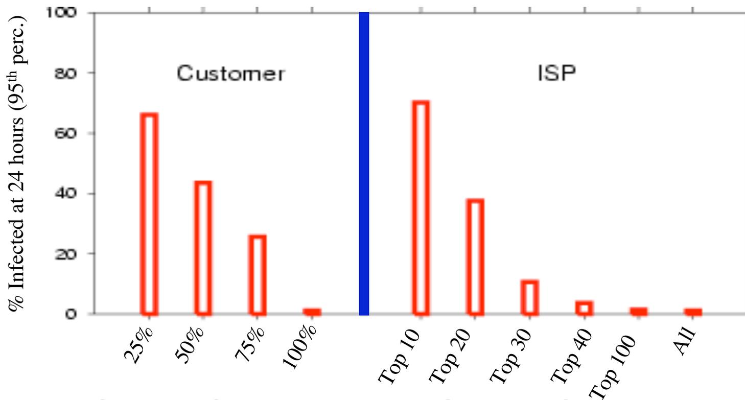
Content filtering firewalls at edge of customer nets.
