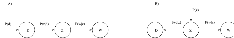
Figure 1: Graphical representation of the aspect model in A) asymmetric and B) symmetric formulations.
