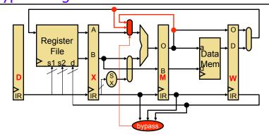
• Each multiplexor has its own, here it is for "ALUinA" (X.IR.RegSrc1 == M.IR.RegDest) => 0 (X.IR.RegSrc1 == W.IR.RegDest) => 1 Else => 2
