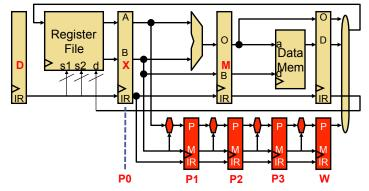
Fix to problem on previous slide: Stall = (OldStallLogic) || ((D.IR.RegDest == X.IR.RegDest) && (X.IR.Operation == MULT))
