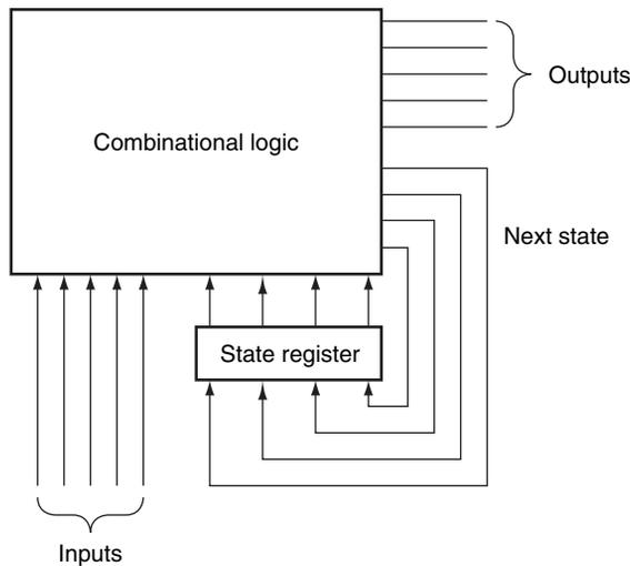
**FIGURE C.10.3** A finite-state machine is implemented with a state register that holds the current state and a combinational logic block to compute the next state and output functions. The latter two functions are often split apart and implemented with two separate blocks of logic, which may require fewer gates.
