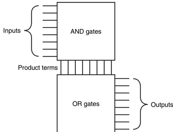
**FIGURE C.3.3** The basic form of a PLA consists of an array of AND gates followed by an array of OR gates. Each entry in the AND gate array is a product term consisting of any number of inputs or inverted inputs. Each entry in the OR gate array is a sum term consisting of any number of these product terms.
