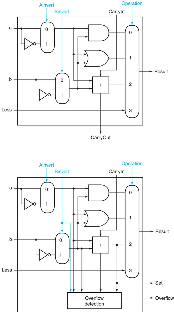
**FIGURE C.5.10 (Top) A 1-bit ALU that performs AND, OR, and addition on a and b or  $\bar{b}$ , and (bottom) a 1-bit ALU for the most significant bit.** The top drawing includes a direct input that is connected to perform the set on less than operation (see Figure C.5.11); the bottom has a direct output from the adder for the less than comparison called Set. (See Exercise C.24 at the end of this Appendix to see how to calculate overflow with fewer inputs.)
