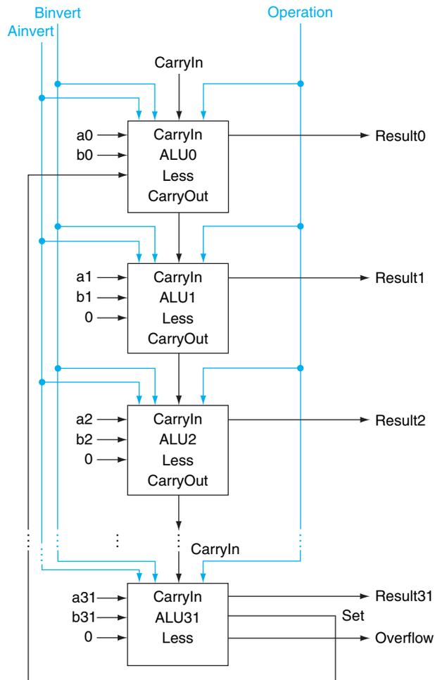
**FIGURE C.5.11** A 32-bit ALU constructed from the 31 copies of the 1-bit ALU in the top of Figure C.5.10 and one 1-bit ALU in the bottom of that figure. The Less inputs are connected to 0 except for the least significant bit, which is connected to the Set output of the most significant bit. If the ALU performs  $a - b$  and we select the input 3 in the multiplexor in Figure C.5.10, then Result = 0 . . . 001 if  $a < b$ , and Result = 0 . . . 000 otherwise.
