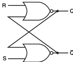
**FIGURE C.8.1** A pair of cross-coupled NOR gates can store an internal value. The value stored on the output  $Q$  is recycled by inverting it to obtain  $\bar{Q}$  and then inverting  $\bar{Q}$  to obtain  $Q$ . If either  $R$  or  $\bar{Q}$  is asserted,  $Q$  will be deasserted and vice versa.
