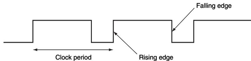
**FIGURE C.7.1** A clock signal oscillates between high and low values. The clock period is the time for one full cycle. In an edge-triggered design, either the rising or falling edge of the clock is active and causes state to be changed.
