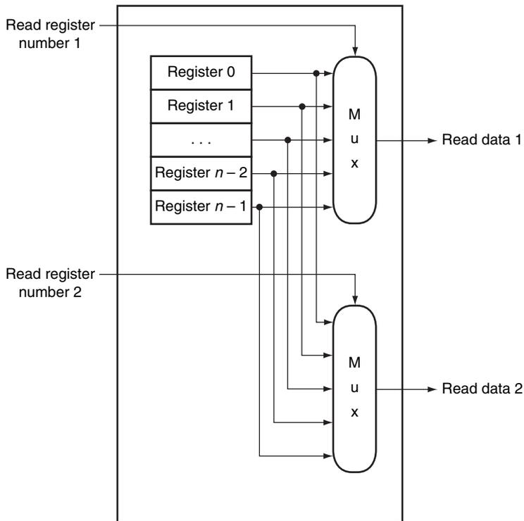
**FIGURE C.8.8** The implementation of two read ports for a register file with  $n$  registers can be done with a pair of  $n$ -to-1 multiplexers, each 32 bits wide. The register read number signal is used as the multiplexor selector signal. Figure C.8.9 shows how the write port is implemented.
