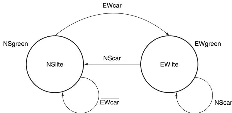
**FIGURE C.10.2** The graphical representation of the two-state traffic light controller. We simplified the logic functions on the state transitions. For example, the transition from NSgreen to EWgreen in the next-state table is  $(\overline{NScar} \cdot EWcar) + (NScar \cdot EWcar)$ , which is equivalent to EWcar.
