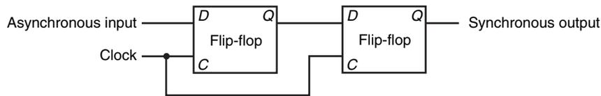
**FIGURE C.11.6** This synchronizer will work correctly if the period of metastability that we wish to guard against is less than the clock period. Although the output of the first flip-flop may be metastable, it will not be seen by any other logic element until the second clock, when the second D flip-flop samples the signal, which by that time should no longer be in a metastable state.
