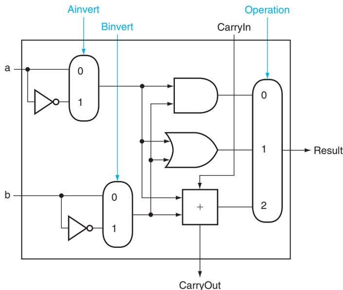
**FIGURE C.5.9** A 1-bit ALU that performs AND, OR, and addition on  $a$  and  $b$  or  $\bar{a}$  and  $\bar{b}$ . By selecting  $\bar{a}$  (Ainvert = 1) and  $\bar{b}$  (Binvert = 1), we get a NOR  $b$  instead of a AND  $b$ .
