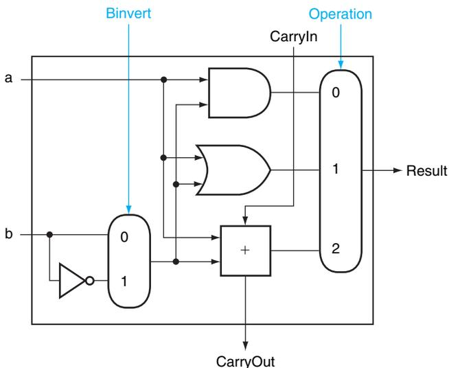
**FIGURE C.5.8** A 1-bit ALU that performs AND, OR, and addition on  $a$  and  $b$  or  $a$  and  $\bar{b}$ . By selecting  $\bar{b}$  (Binvert = 1) and setting CarryIn to 1 in the least significant bit of the ALU, we get two's complement subtraction of  $b$  from  $a$  instead of addition of  $b$  to  $a$ .
