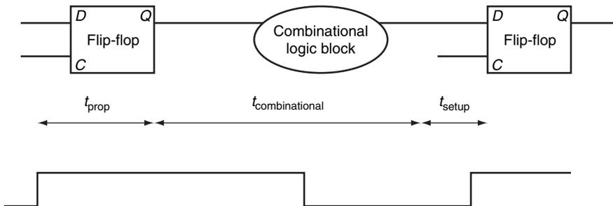
**FIGURE C.11.1** In an edge-triggered design, the clock must be long enough to allow signals to be valid for the required setup time before the next clock edge. The time for a flip-flop input to propagate to the flip-flop outputs is  $t_{\text{prop}}$ ; the signal then takes  $t_{\text{combinational}}$  to travel through the combinational logic and must be valid  $t_{\text{setup}}$  before the next clock edge.
