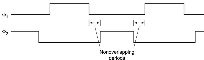
**FIGURE C.11.3** A two-phase clocking scheme showing the cycle of each clock and the nonoverlapping periods.
