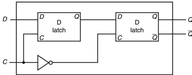
**FIGURE C.8.4** A D flip-flop with a falling-edge trigger. The first latch, called the master, is open and follows the input  $D$  when the clock input,  $C$ , is asserted. When the clock input,  $C$ , falls, the first latch is closed, but the second latch, called the slave, is open and gets its input from the output of the master latch.
