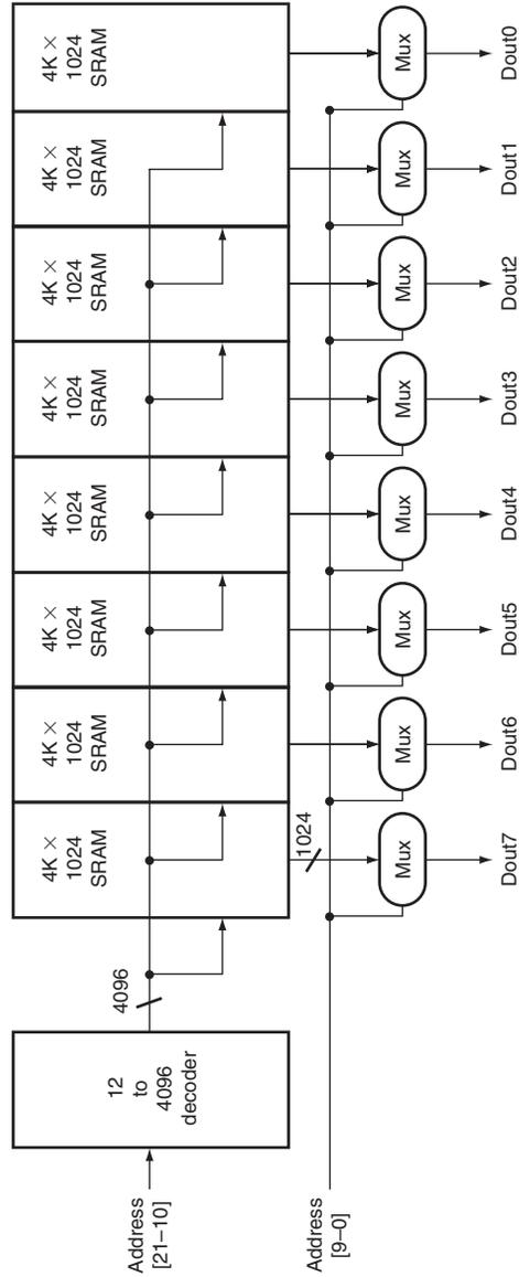
**FIGURE C.9.4 Typical organization of a 4M x 8 SRAM as an array of 4K x 1024 arrays.** The first decoder generates the addresses for eight 4K x 1024 arrays; then a set of multiplexers is used to select 1 bit from each 1024-bit-wide array. This is a much easier design than a single-level decode that would need either an enormous decoder or a gigantic multiplexor. In practice, a modern SRAM of this size would probably use an even larger number of blocks, each somewhat smaller.
