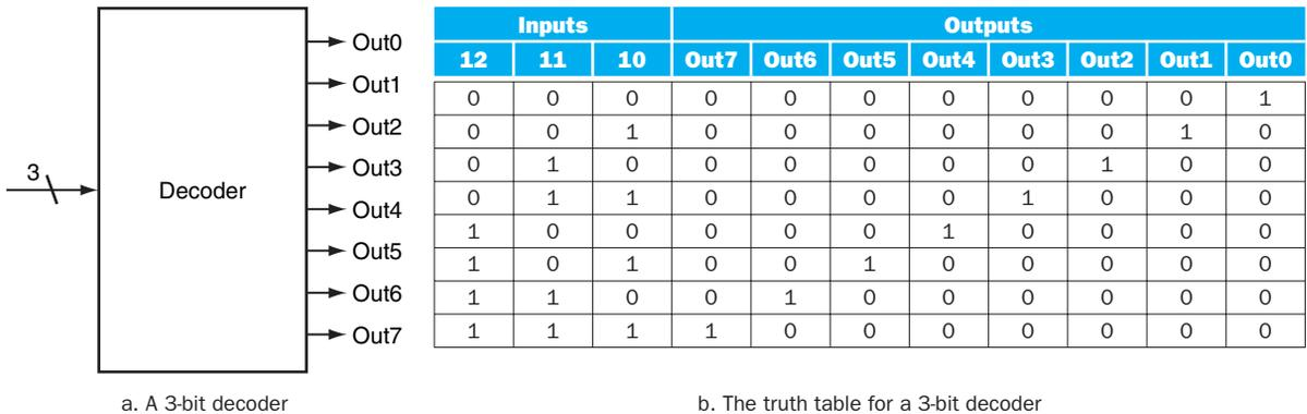
**FIGURE C.3.1** A 3-bit decoder has 3 inputs, called 12, 11, and 10, and  $2^3 = 8$  outputs, called Out0 to Out7. Only the output corresponding to the binary value of the input is true, as shown in the truth table. The label 3 on the input to the decoder says that the input signal is 3 bits wide.
