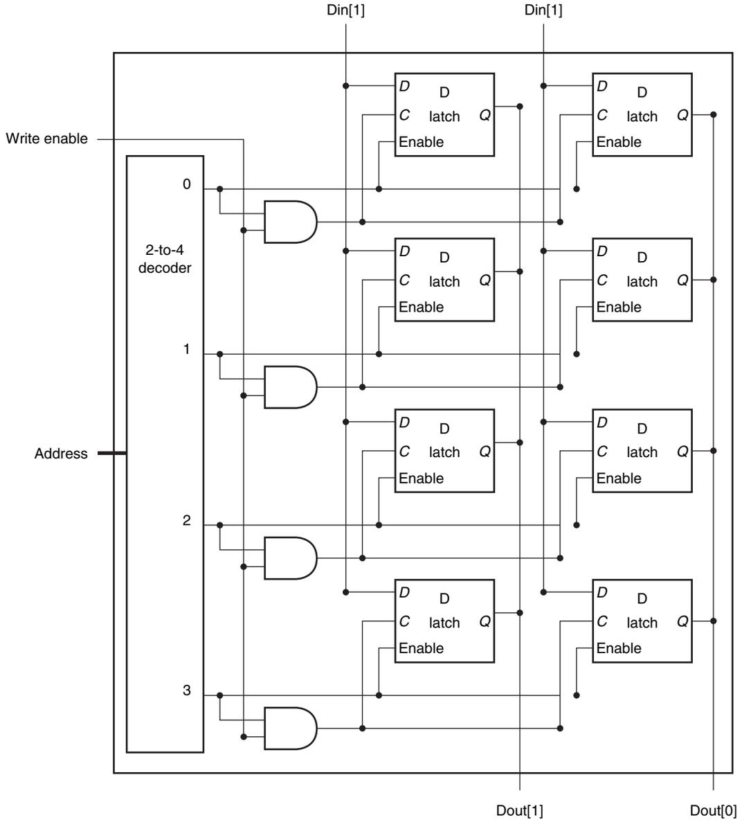
**FIGURE C.9.3** The basic structure of a  $4 \times 2$  SRAM consists of a decoder that selects which pair of cells to activate. The activated cells use a three-state output connected to the vertical bit lines that supply the requested data. The address that selects the cell is sent on one of a set of horizontal address lines, called word lines. For simplicity, the Output enable and Chip select signals have been omitted, but they could easily be added with a few AND gates.
