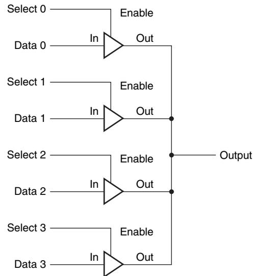
**FIGURE C.9.2** Four three-state buffers are used to form a multiplexer. Only one of the four Select inputs can be asserted. A three-state buffer with a deasserted Output enable has a high-impedance output that allows a three-state buffer whose Output enable is asserted to drive the shared output line.
