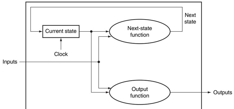
**FIGURE C.10.1** A state machine consists of internal storage that contains the state and two combinational functions: the next-state function and the output function. Often, the output function is restricted to take only the current state as its input; this does not change the capability of a sequential machine, but does affect its internals.
