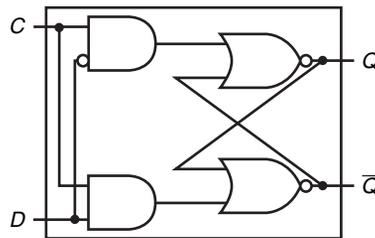
**FIGURE C.8.2 A D latch implemented with NOR gates.** A NOR gate acts as an inverter if the other input is 0. Thus, the cross-coupled pair of NOR gates acts to store the state value unless the clock input,  $C$ , is asserted, in which case the value of input  $D$  replaces the value of  $Q$  and is stored. The value of input  $D$  must be stable when the clock signal  $C$  changes from asserted to deasserted.
