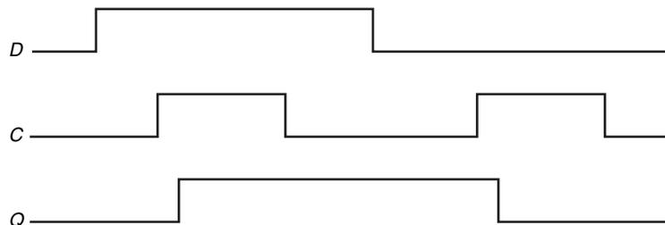
**FIGURE C.8.3 Operation of a D latch, assuming the output is initially deasserted.** When the clock,  $C$ , is asserted, the latch is open and the  $Q$  output immediately assumes the value of the  $D$  input.
