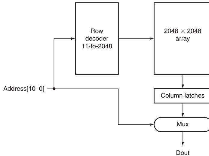
**FIGURE C.9.6** A  $4\text{M} \times 1$  DRAM is built with a  $2048 \times 2048$  array. The row access uses 11 bits to select a row, which is then latched in 2048 1-bit latches. A multiplexor chooses the output bit from these 2048 latches. The RAS and CAS signals control whether the address lines are sent to the row decoder or column multiplexor.
