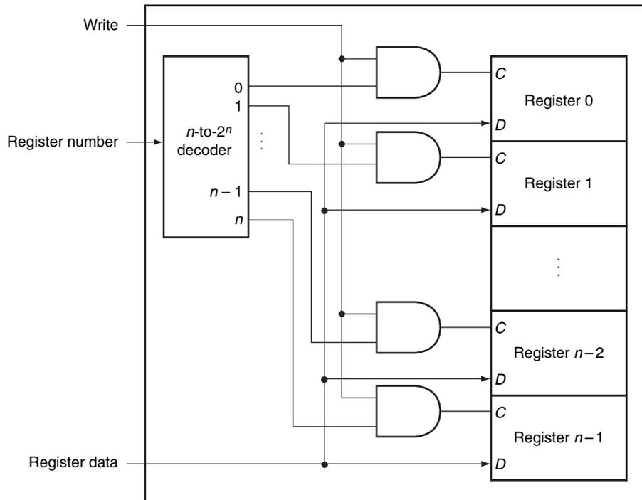
**FIGURE C.8.9** The write port for a register file is implemented with a decoder that is used with the write signal to generate the  $C$  input to the registers. All three inputs (the register number, the data, and the write signal) will have setup and hold-time constraints that ensure that the correct data is written into the register file.
