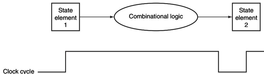
**FIGURE C.7.2** The inputs to a combinational logic block come from a state element, and the outputs are written into a state element. The clock edge determines when the contents of the state elements are updated.
