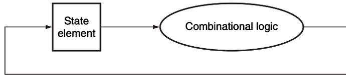
**FIGURE C.7.3** An edge-triggered methodology allows a state element to be read and written in the same clock cycle without creating a race that could lead to undetermined data values. Of course, the clock cycle must still be long enough so that the input values are stable when the active clock edge occurs.
