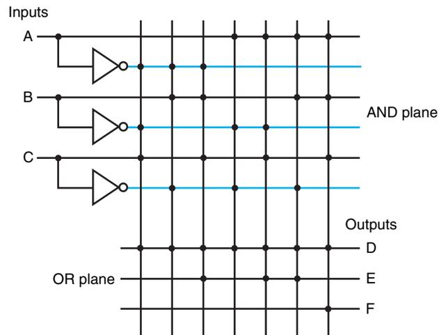
**FIGURE C.3.5 A PLA drawn using dots to indicate the components of the product terms and sum terms in the array.** Rather than use inverters on the gates, usually all the inputs are run the width of the AND plane in both true and complement forms. A dot in the AND plane indicates that the input, or its inverse, occurs in the product term. A dot in the OR plane indicates that the corresponding product term appears in the corresponding output.
