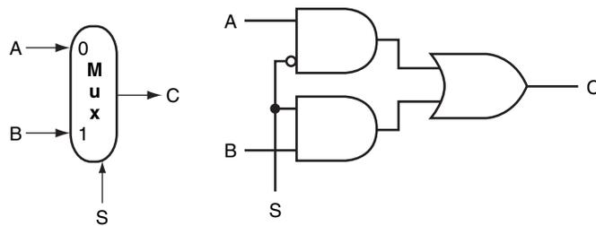
**FIGURE C.3.2** A two-input multiplexor on the left and its implementation with gates on the right. The multiplexor has two data inputs ( $A$  and  $B$ ), which are labeled  $0$  and  $1$ , and one selector input ( $S$ ), as well as an output  $C$ . Implementing multiplexors in Verilog requires a little more work, especially when they are wider than two inputs. We show how to do this beginning on page C-23.
