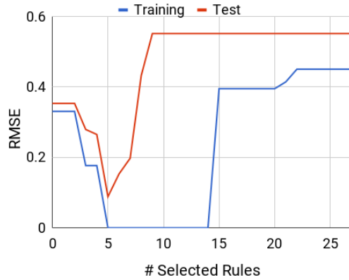
Figure 3: Training and test RMSE as a function of number of selected rules from the DIFFLOG program.
