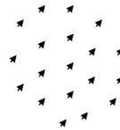
Using Artificial Physics, MAVs form a hexagonal lattice sensing grid
