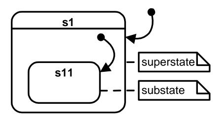
The substates need only define the differences from the superstates, and otherwise can easily share (reuse) behavior defined in higher levels of nesting
