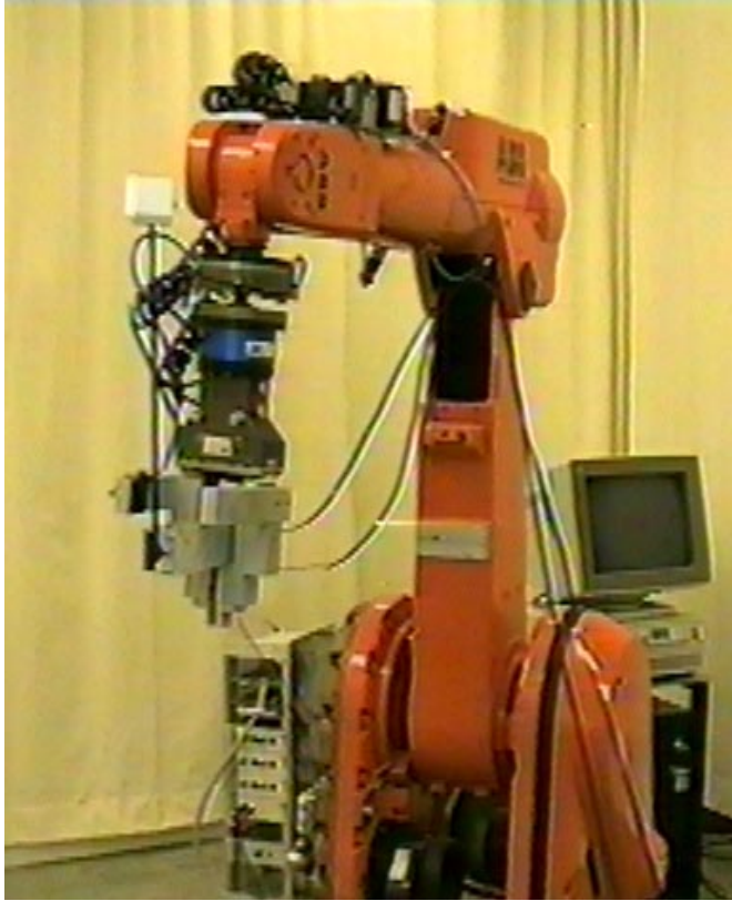
Figure 3. The ABB Irb2000 robot and the pendulum used in the experiment.
