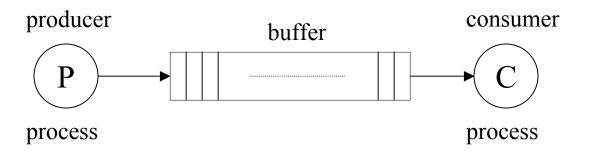
from time to time, the producer places an item in the buffer the consumer removes an item from the buffer careful synchronization required the consumer must wait if the buffer empty the producer must wait if the buffer full typical solution would involve a shared variable count also known as the Bounded Buffer problem Example: in UNIX shell
