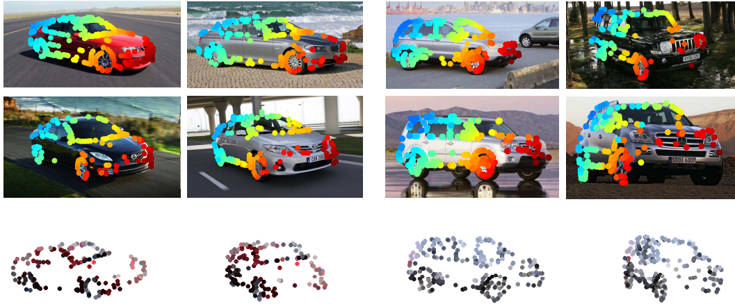
Figure 6. Matching different cars. Best viewed in color. Left: the correspondences of sedan images and the reconstruction. Right: the correspondences of SUV images and the reconstruction. Only four selected images are shown for each image set. Note that the cars in images are all different and the feature points are automatically detected. The markers with the same color indicate the matched feature points. The 3D reconstruction is rendered with the colors in the first image and visualized in two viewpoints.
