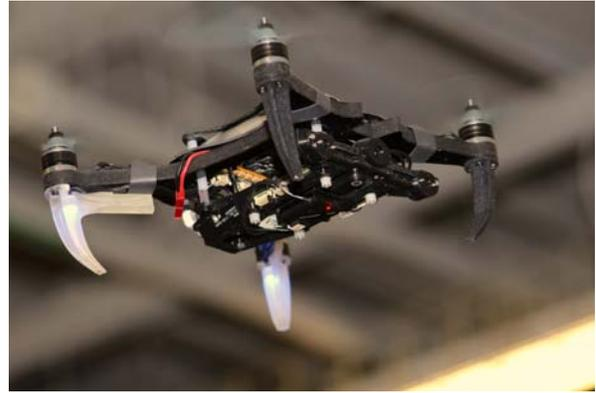
Fig. 1. A 22 cm, 250 g quadrotor with a forward-facing stereo camera pair.
