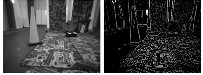
Fig. 3. The left image shows the grayscale image, and the right image shows only the high gradient pixels selected by the system.
