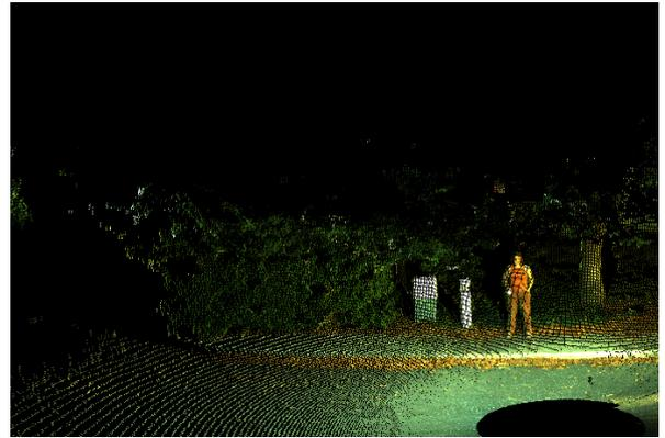
Fig. 7. A LIDAR scan colored using camera pixels.
