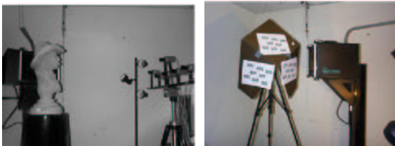
Figure 6. Experimental Setup: Buffalo Bill statue, scanner head and camera cluster (left), 3D target for coordinate frame registration (right).
