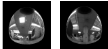
Figure 5: Rotated Images. Two spherical images from a sequence of catadioptric images rotated relatively about the mirror’s optical axis.
