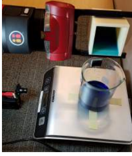
Fig. 4: We use the Rethink Robotics Sawyer manipulator to precisely pour colored water into a beaker using visual feedback from a mvBluefox MLC202bc camera.
