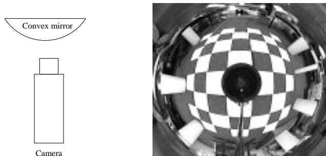
Figure 2. On the left we see one way to create a panoramic sensor: point a camera upwards at a curved mirror. On the right we see an image from such a panoramic sensor, with the camera visible in the center.
