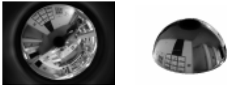
Figure 1. On the left a parabolic catadioptric image; on the right its 1:1 mapping to a hemi-sphere.
