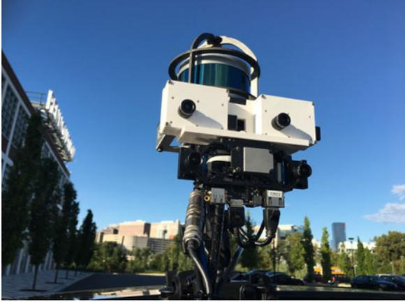
Fig. 1. Full sensor rig, with stereo DAVIS cameras, VI Sensor and Velodyne lidar.
