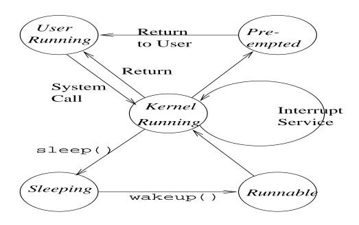
Figure 1: UNIX processes: An abstract state diagram
