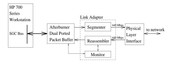
Figure 3: ATM Link Adapter
