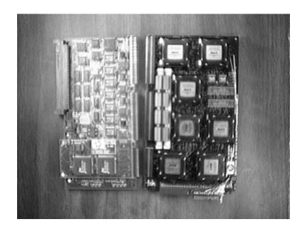
Figure 2: Afterburner (left) and ATM Link Adapter (right)
