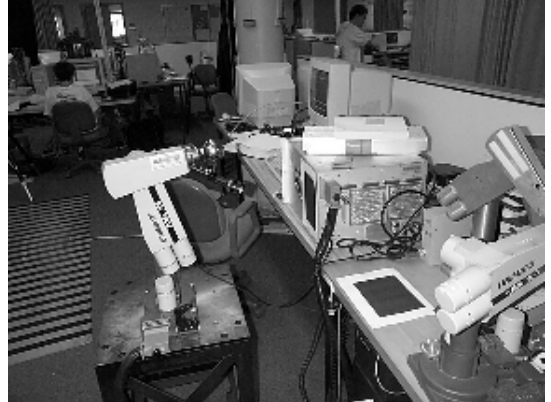
Figure 3: Pose control experiments were carried out on a Puma 260 robot arm outfitted with a video camera.
