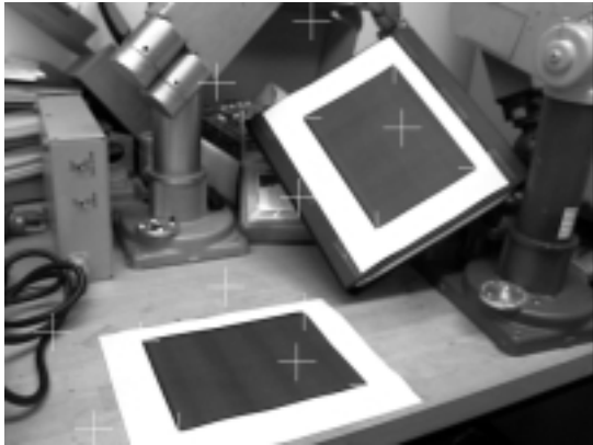
Figure 4: This figure shows an image obtained from the camera mounted on the robot arm. The relative orientation of the camera with respect to the target position was obtained by tracking the corners of the black rectangles in the image. The white crosses are used to mark both the current locations of these features in this image and the target image configuration.
