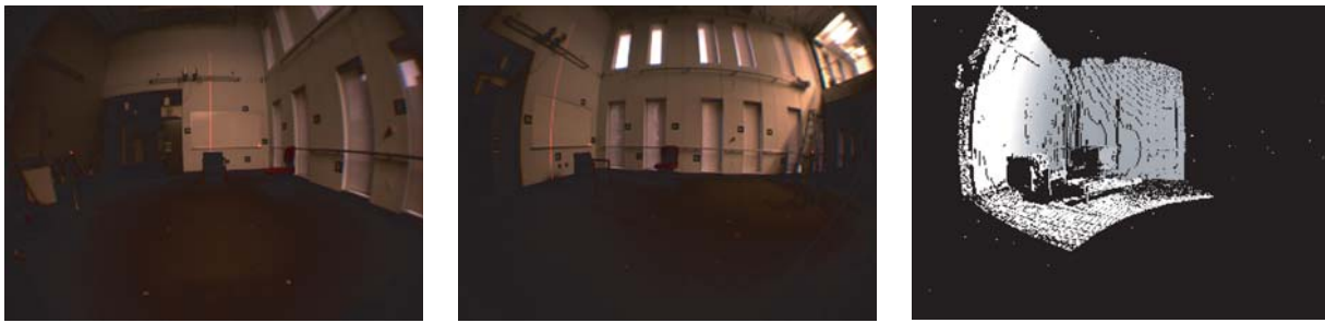
Figure 6. ((a) and (b) show Two images of a scene illuminated with a plane of laser light which is used to establish correspondences between the two views (c) shows the range map constructed based on the correspondences derived from a sequence of such images.
