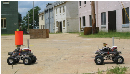
Fig. 3. Two Clodbusters in a Leader-Follower formation. The robot on the left is tele-operated while the robot on the right is executing the blob follower behavior.
