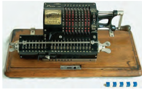
Figure 9. Dactyle calculator based on the pinwheel design of the Russian-Swedish entrepreneur Willgodt Odhner. Dactyle resold machines made by Brunsviga in Braunschweig and from 1905 by Chateau Bros. in Foncine-le-Haut.
