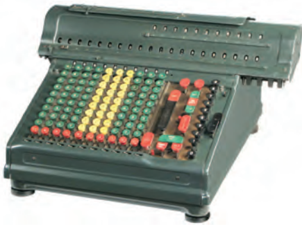
Figure 11. Crout's method was performed with machines such as this Marchant calculator, model 10ACT. It was manufactured in Oakland, California, in the 1930s and 1940s.
