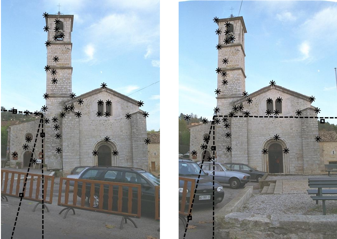
Figure 4.13: Results of fundamental matrix estimation for the Valbonne sequence. The 45 inliers returned by pbM and epipolar lines of the 3 outliers misclassified as inliers are shown.
