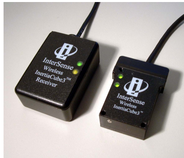
Figure 5.4: Wireless Inertia Cube 3 and the wireless receiver.
