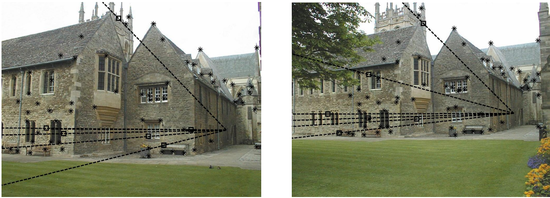
Figure 4.11: Results of fundamental matrix estimation for the Merton College images. The 68 inliers returned by pbM and epipolar lines of the 6 outliers misclassified as inliers are shown. The reason for the misclassifications is explained in the text.
