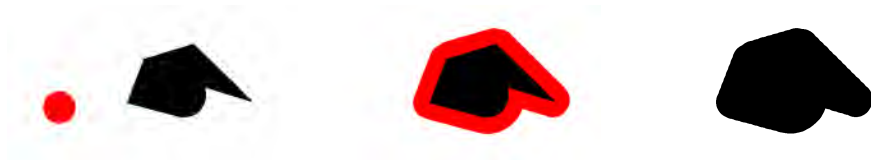
Fig. 3.28 Illustration of shape offsetting. Starting from the black set A and the red ball B (left), \delta_B A is constructed (middle and right.)
