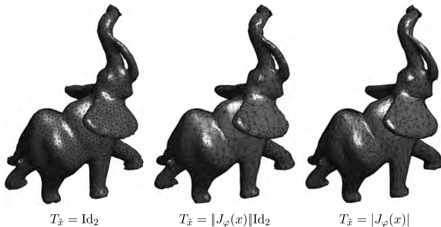
Fig. 4.16 Comparison of constant, isotropic and anisotropic surface remeshing, with N = 3200 points.
