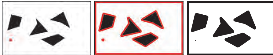
Fig. 3.30 Illustration of shape offsetting. Assuming one wants to compute the trajectory of a circular object in an environment \Omega with obstacles (top), one can grow the obstacles, leading to a new environment \Omega' (middle), and the problem is thus reduced to computing the trajectory of a point in the obtained space (right).
