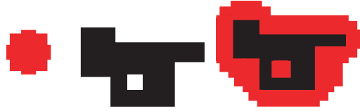
Fig. 2.20 Discrete dilation of the black shape S_d by the red kernel B_d .
