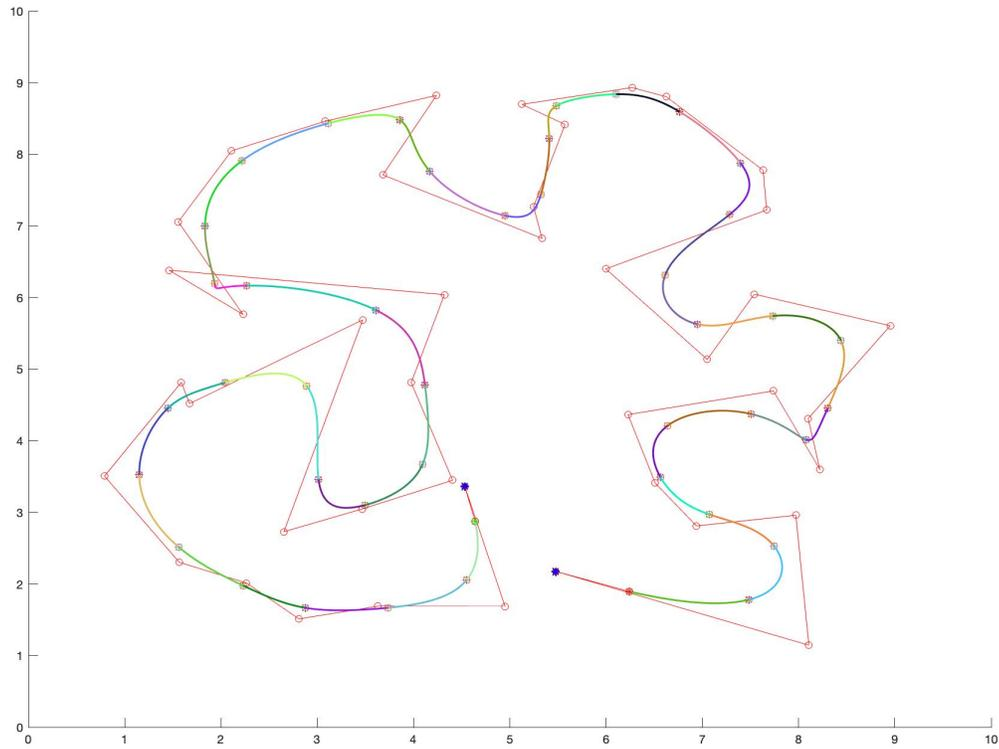
Figure 11: A quintic interpolating  $B$ -spline for 43 data points.
