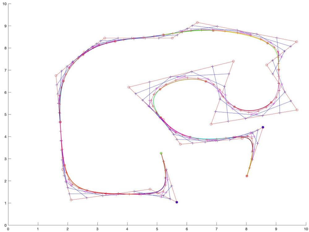
Figure 3: A quintic interpolating  $B$ -spline for 22 data points.
