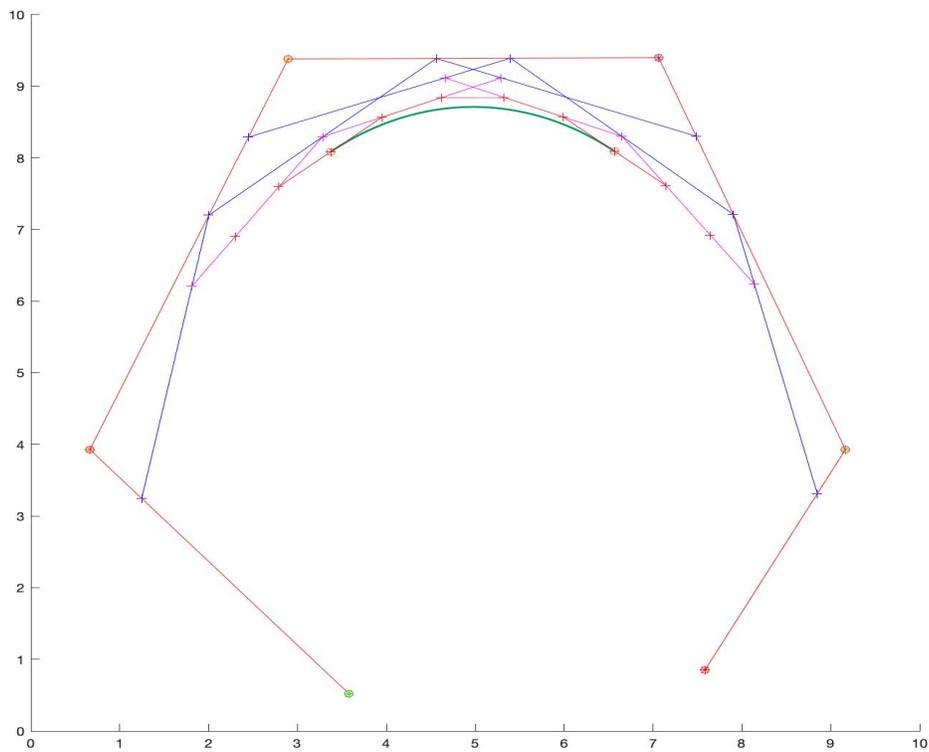
Figure 5: Construction of a generic quintic Bézier curve.
