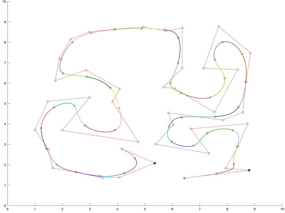
Figure 4: A quintic interpolating  $B$ -spline for 44 data points.
