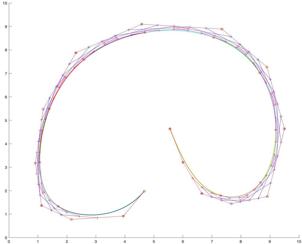
Figure 6: A quintic  $B$ -spline with 16 de Boor control points.
