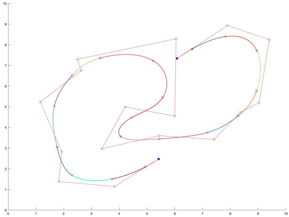
Figure 9: A quintic interpolating  $B$ -spline for 18 data points.
