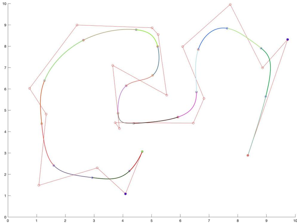
Figure 2: A quintic interpolating  $B$ -spline for 20 data points.
