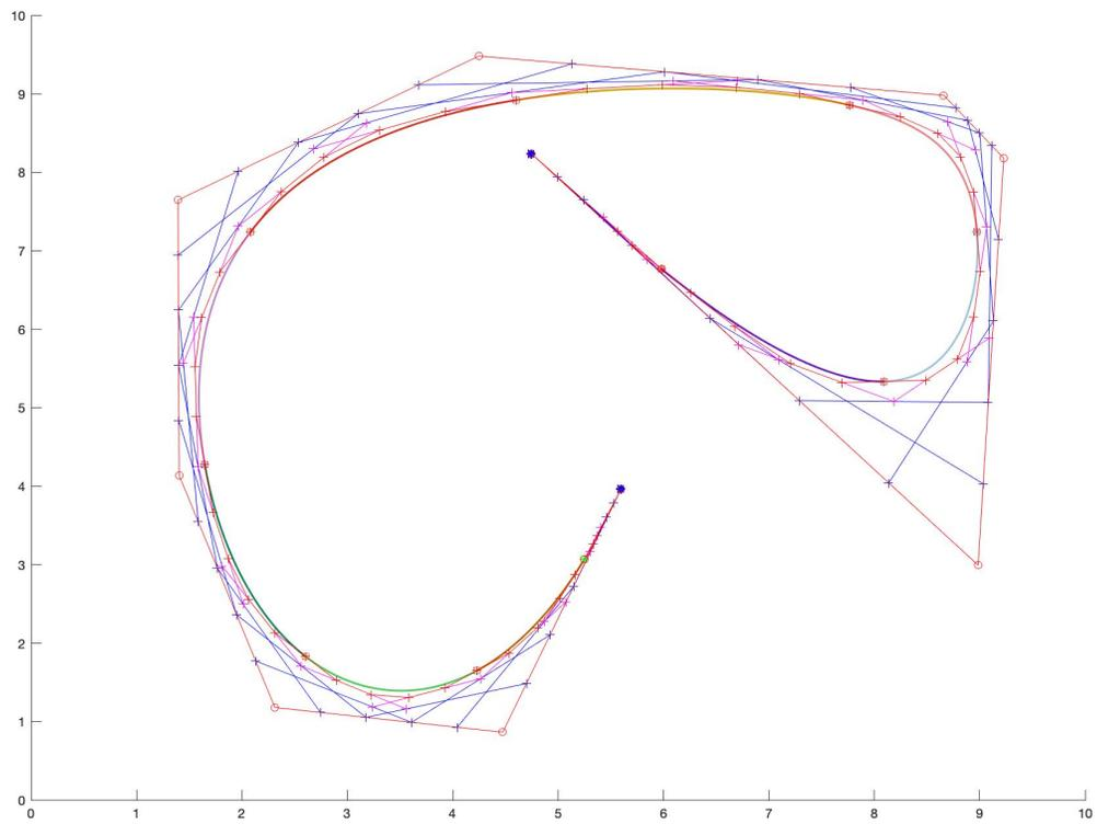
Figure 10: A quintic interpolating  $B$ -spline for 10 data points.
