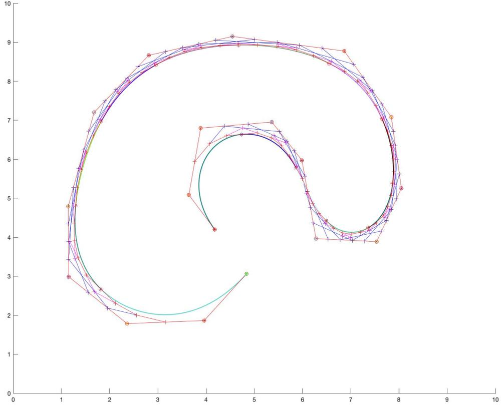
Figure 7: A quintic  $B$ -spline with 18 de Boor control points.
