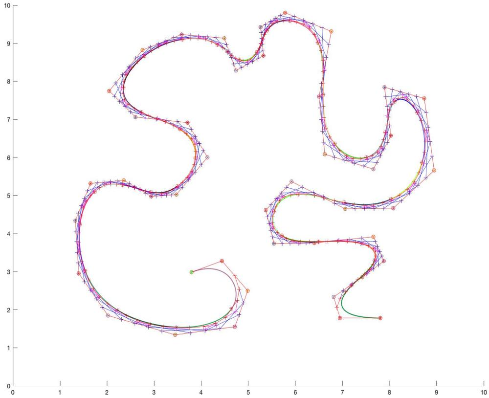
Figure 8: A quintic  $B$ -spline with 43 de Boor control points.
