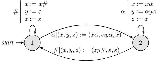
Here  $\alpha \in \{a, b\}$  and the output function  $F$  is defined by  $F(\{2\}) = x$ .
