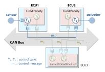
Figure 14: System architecture for the lane keeping system.
