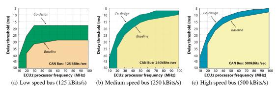
Figure 16: ECU1 design feasibility regions with respect to different bus speed values.
