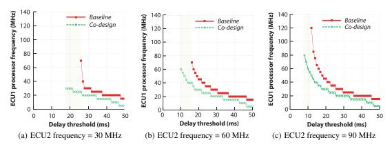
Figure 15: ECU1 processor frequency for different delay thresholds.
