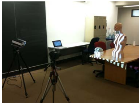
Figure 1. In a structured light system the scene is illuminated by a projector and the images are captured with a camera.
