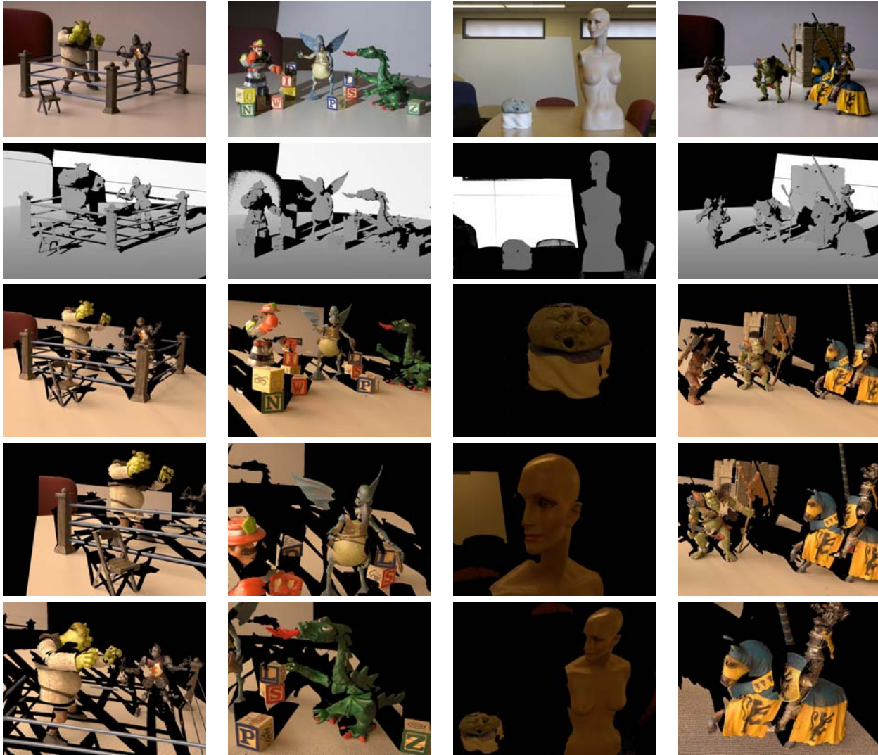
Figure 10. This figure shows results obtained by applying the proposed reconstruction scheme to a few different scenes. The first row corresponds to the original input image. The second row depicts the recovered depth map and the remaining 3 rows show novel views of the scene produced using a splatting renderer.
